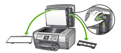
2. Unfold the holder so that the half with four slide openings is on top.
