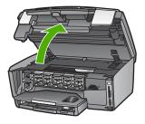
Squeeze the tab below an ink cartridge to release the latch inside the HP All-in-One; then lift the latch.
