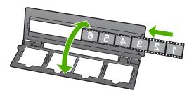
4. Place the holder on the glass and match the bottom edge with the bottom edge of the glass. Then, match the right tab on the top half of the holder with the right edge of the glass.
