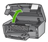
2. Squeeze the tab below an ink cartridge to release the latch inside the HP All-in-One, and then lift the latch.
