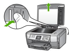
4. When you finish copying or scanning, replace the lid by inserting the tabs on the hinge back into the appropriate slots, and then reconnect the Slide and Negative light power cord. Replace the cord in the cord clips on the back of the HP All-in-One.
