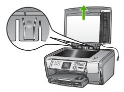
3. Press the hinge releases until the lid separates from the rest of the HP All-in-One.
