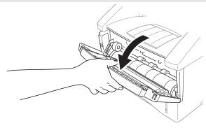
**3** Insert the drum unit assembly into the machine.
