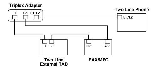
You can keep two-line telephones on other wall outlets as always. There are two ways to add a two-line telephone to the machine's wall outlet. You can plug the telephone line cord from the two-line telephone into the L1+L2 jack of the triplex adapter. Or, you can plug the two-line telephone into the TEL jack of the two-line TAD.
