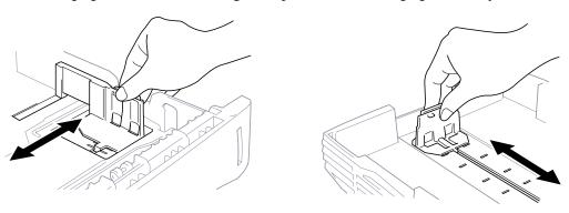
Fan the paper well. Load paper in the paper cassette. Press down on the paper to flatten it in all four corners, keeping the paper level below the guide. The cassette can hold up to 250 sheets of 20 lb (75g/m²) paper.
