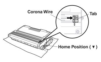
**8** Reinstall the drum unit and close the front cover.
