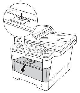
3 Slowly take out the drum unit and toner cartridge assembly. The jammed paper may be pulled out with the drum unit and toner cartridge assembly, or this may release the paper so you can pull it out from inside of the machine.
