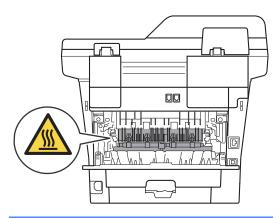
5 Pull the green tabs at the left and right hand sides toward you and fold down the fuser cover (1).
