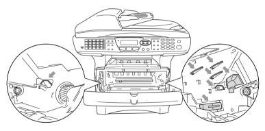
**3** Hold down the lock lever on the right and pull the toner cartridge out of the drum unit. (See *Replacing the toner cartridge* on page 12-27.)
