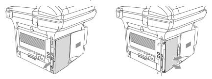
**3** Loosen the two screws, and then remove the metal cover plate.
