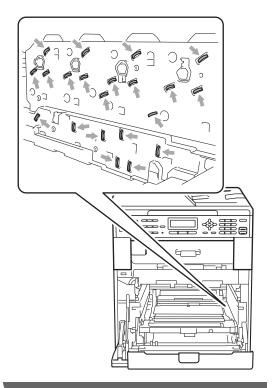
5 Hold the green handle of the belt unit with both hands and lift the belt unit up, then pull it out.
