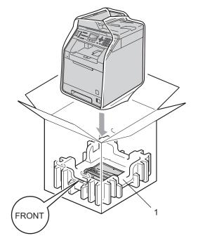
Put the two styrofoam pieces (1) into the carton matching the right of the machine to the "RIGHT" mark on one of the styrofoam pieces, and the left of the machine to the "LEFT" mark on the other styrofoam piece. Put the AC power cord and printed materials in the original carton as shown in the illustration.
