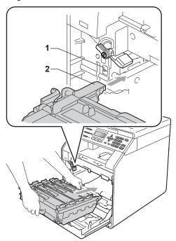
Turn the green lock lever (1) clockwise to the lock position.
