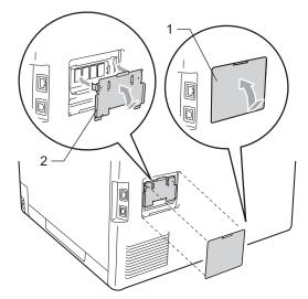
Plug the machine's power cord back into the electrical socket first, and then connect the interface cable.
