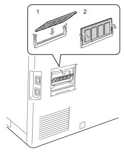
6 Put the metal (2) and then the plastic (1) SO-DIMM covers back on.
