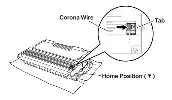
**8** Reinstall the drum unit into the machine and close the front cover.
