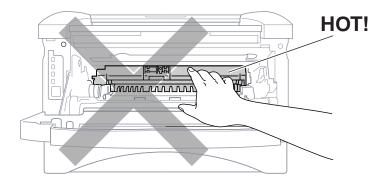
Open the front cover and pull out the drum unit.
