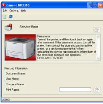
If the service error appears, cycle the power of the printer using the following procedure. This may clear the message.
