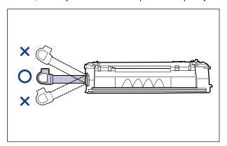
• Pull out the sealing tape completely from the toner cartridge. If any tape remains in the toner cartridge, this may result in poor print quality.
