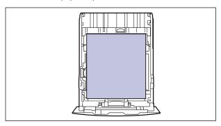
• If you use paper that has been poorly cut, multiple sheets of paper may be fed at once. In this case, align the edges of the paper stack properly on a hard, flat surface.
