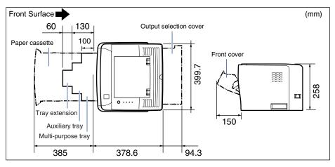
• With the paper feeder installed
