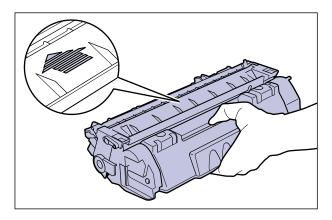
3. Push the toner cartridge into the printer firmly until it touches the back of the printer while aligning (A) on both sides of the toner cartridge with the toner cartridge guides inside the printer.
