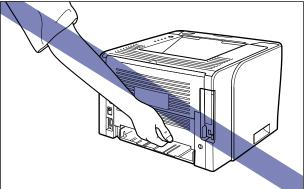
• The rear portion (A) of the printer is relatively heavy. Be careful not to become off-balance when lifting the printer. If you do so, you may drop the printer, resulting in personal injury.
