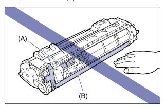
• Be careful not to hold or touch areas that are not specified in this procedure, such as the electrical contacts (C). This may result in damage to the cartridge.
