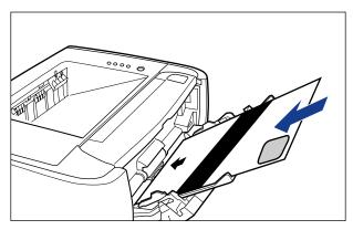
The paper is fed into the printer slowly, and the printer starts cleaning the fixing roller.
