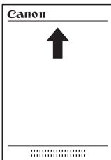
**When setting an envelope, gently insert the envelope into the multi-purpose tray with the print side up and the right edge (i.e., closer to the stamp) first.**
