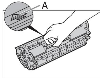
**7 Insert the cartridge so that the protrusion on the right side of the toner cartridge (A) fits into the guide (B) located on the right side of the machine and slide it down parallel to the guide.**
