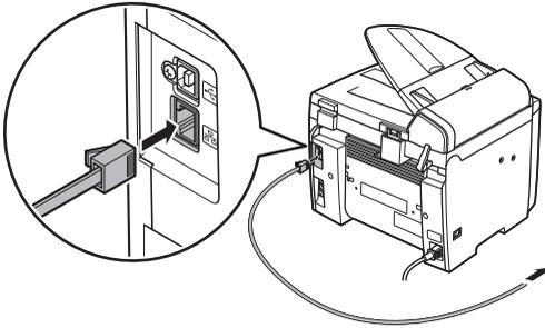
**Set up the machine for use in a network, then connect the machine and the PC to your network router or a hub.**
