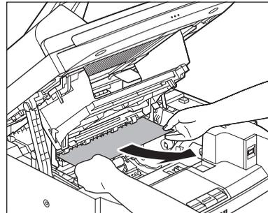
**5** Gently pull the jammed paper between the fixing assembly (A) and transfer roller (B) until the leading edge emerges from the machine.
