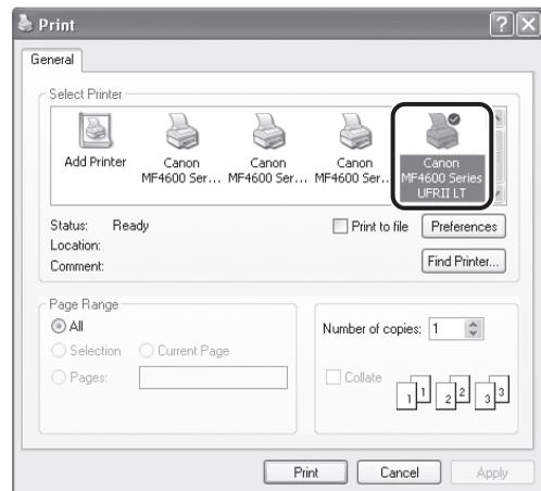
Select the printer icon for the machine ([Canon MF4600 Series UFR II LT], [Canon MF4600 Series PCL5e], [Canon MF4600 Series PCL6]), then click [Preferences] or [Properties] to open the dialog box.
