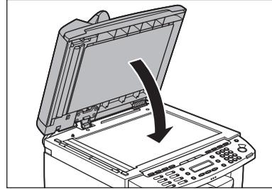
**6** Clean the ADF scanning area (on the left side of the platen glass) with a cloth dampened with water. Then wipe the area with a soft, dry cloth.
