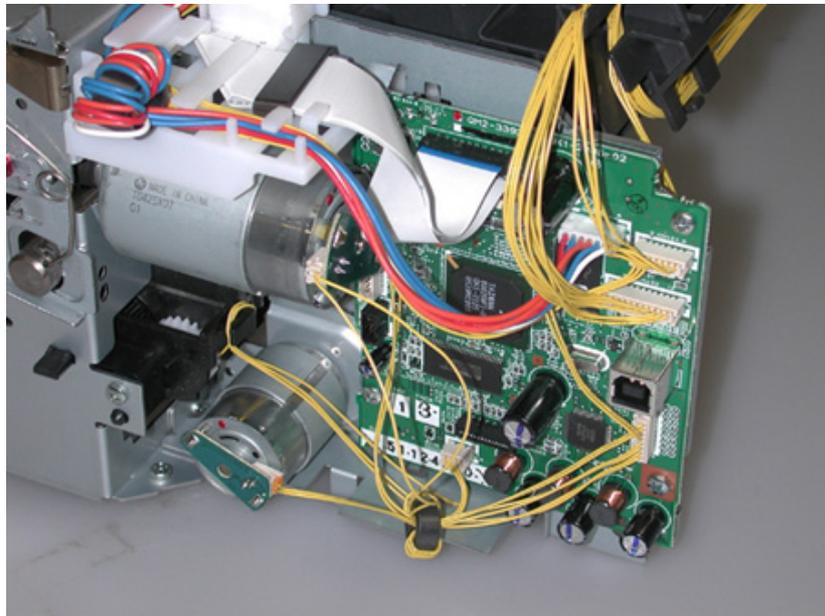
(II) Paper feed motor side wiring
