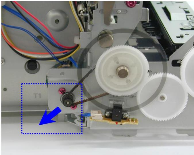
Note: The red screws securing the paper feed motor may be loosened only at replacement of the paper feed motor unit. DO NOT loosen them in other cases.
