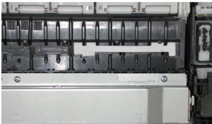
(III) Confirm that the ink absorbers come out from the slots under the output support unit (indicated by the blue circles in the photo below), then peel off the adhesive cover sheet, and attach the ink absorbers to the output support unit as shown in the photo.
