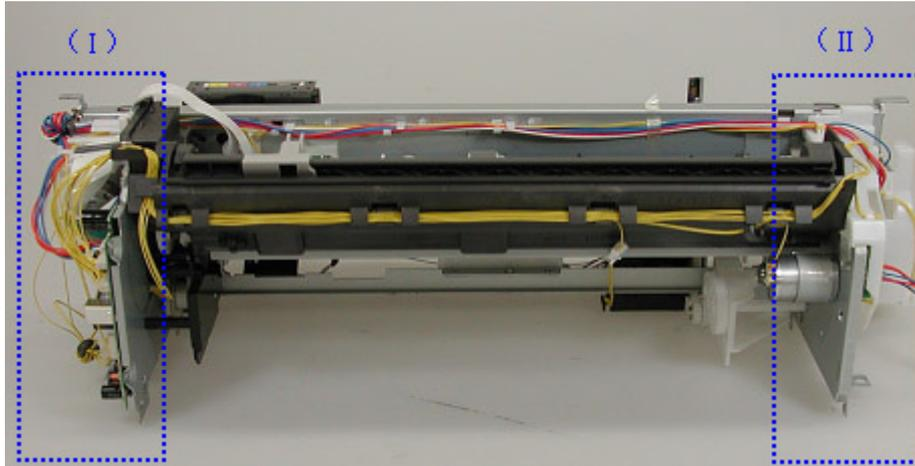
(I) Logic board ass'y wiring
