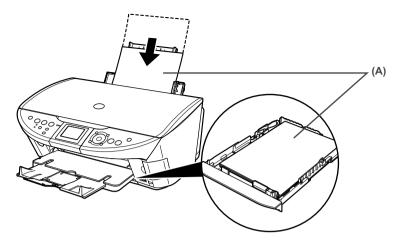
(A) If the Auto Sheet Feeder runs out of paper, the paper source automatically changes to the Cassette.
