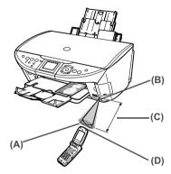
(2) Select the photo to print and send the data to the machine using the infrared communication function of the mobile phone. Printing will start after receiving all data.
