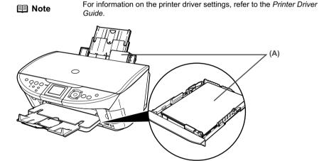
(A) You can switch between paper loaded in the Auto Sheet Feeder (e.g.,  $4" \times 6" / 101.6 \times 152.4$  mm) or the Cassette (e.g., A4/Letter-sized paper).
