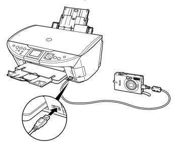
(3) Turn on and set up the device for direct printing. Either of the following icons will display on the LCD display of the device when the machine is correctly connected.
