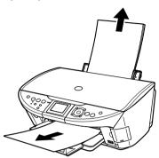
If the paper tears and a piece remains inside the machine, open the Scanning Unit (Printer Cover) and remove it. Be careful not to touch the components inside the machine at this time.
