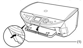
2 Raise the Scanning Unit (Printer Cover) until it stops.
