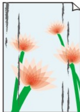
Printed Surface Is Smudged
