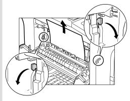
• If the jammed paper is badly folded, similar to the folds of an accordion, ease the jammed paper loose and then pull it out of the printer.
