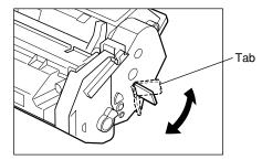
**b** While grasping the cartridge with one hand, firmly and slowly pull the sealing tape tab straight out with the other hand to remove the sealing tape completely. Throw the tape away.
