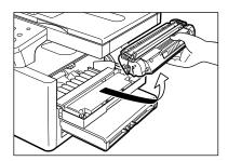
• Don't expose the cartridge to light for more NOTE than 5 minutes. If necessary, put the cartridge in its original protective bag or wrap it with a thick cloth to prevent exposure to light.
