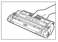
8 Align the projections (A) on both sides of the cartridge to the guides (B) in the machine (location ①) and gently slide the cartridge into the machine until the right cover slightly rises up (location ②).
