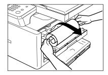
• Do not pull the jammed paper upward; the toner on the paper will stain the printer and cause a permanent reduction in print quality.
