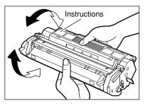
**5** Place the cartridge on a flat and stable surface. Grip the sealing tape tab and snap it in the direction as shown below. Make sure that the tab itself is detached from the cartridge.
