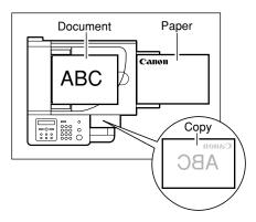
When you place the document on the platen glass, the orientation of the document and the orientation of the paper in the cassette or in the multi-purpose tray are as shown below.
