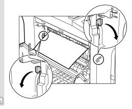
7 Gently pull the jammed paper between the output rollers until the leading edge emerges from the machine.
