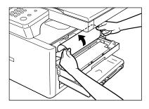
5 If the leading edge of the paper is visible but has not entered the imaging area, pull the paper forwards and roll it inwards.
