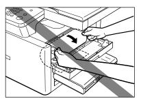
4 Roll the trailing edge of the paper so that the printed surface is on the inside of the roll, then gently pull the rolled up paper out of the machine.
