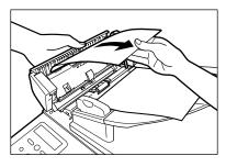
2 Widen the slide guides until they stop, remove the paper so as not to be caught by the slide guides. Open the ADF and gently remove the jammed paper from the ADF.
