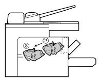
• If the LCD displays INSTALL CARTRIDGE, reset the machine by opening the right cover and then closing it.
