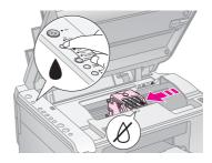
If none of the cartridges are low or empty, the print head moves to the ink cartridge replacement position. Go to step 5.
