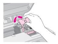
Squeeze the tab at the back of the empty/low cartridge and lift it straight out. Dispose of it carefully. Do not take the used cartridge apart or try to refill it.
