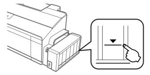
☐ The L1300 has two black ink tanks. Make sure the ink level for both ink tanks is above the lower line.
