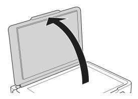
Use a soft, dry, clean cloth to clean the surface of the scanner glass.
