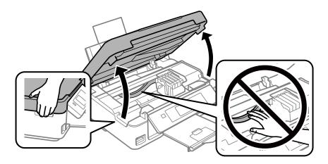
3. Check if the translucent film is smeared. Smears are easier to see if you use a light. If there are smears (such as finger marks or grease) on the translucent film (A), go to the next step.
