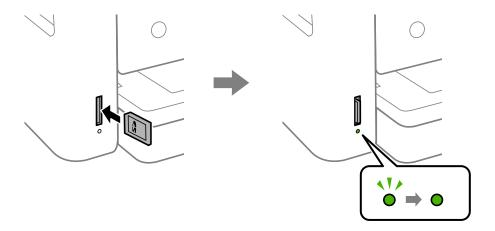
2. When you have finished using the memory card, make sure the light is not flashing, and then push the card to remove it.
