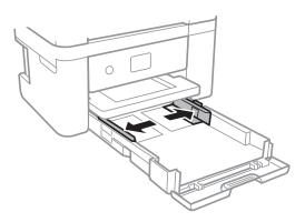
4. With the printable side facing down, load paper until it touches the back of the paper cassette.
