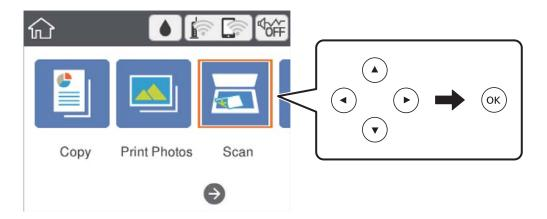
Move the focus to the setting item using the  $\blacktriangle$   $\blacktriangledown$   $\blacktriangleleft$  buttons, and then press the OK button to switch the item on or off.
