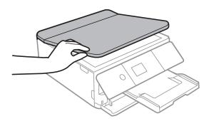
2. Use a soft, dry, clean cloth to clean the surface of the scanner glass.
