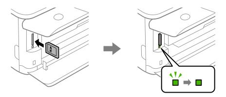
3. When you have finished using the memory card, make sure the light is not flashing, and then push the card to remove it.
