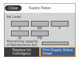
You can check the approximate ink levels and the approximate service life of the maintenance box. You can also replace the ink cartridges or print the supply status information.
