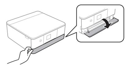
3. Check that the printer is not operating, and then slide out the paper cassette 1.
