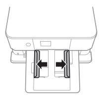
5. With the printable side facing down, load paper until it touches the back of paper cassette 1.
