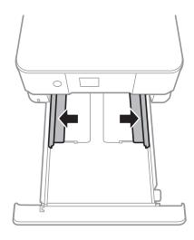
5. With the printable side facing down, load paper until it touches the back of paper cassette 2.
