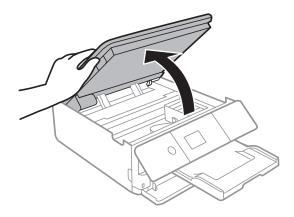
3. Check if the translucent film is smeared. Smears are easier to see if you use a light. If there are smears (such as finger marks or grease) on the translucent film (A), go to the next step.
