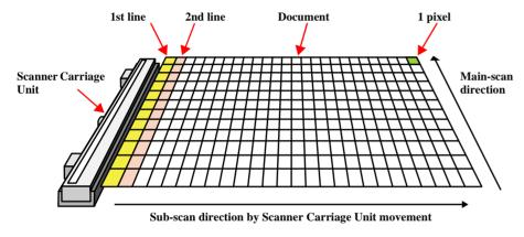
Figure 2-15. Scanner Carriage Unit Movement
