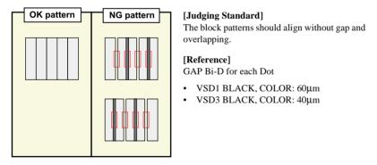
Figure 5-3. Bi-D Adjustment Printing Pattern
