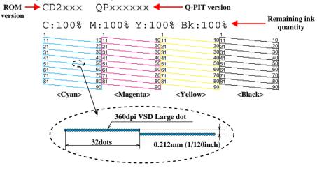
Figure 1-24. Nozzle check pattern
