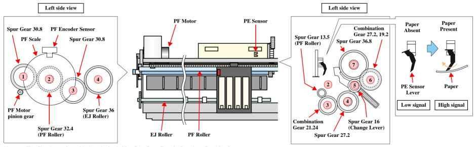
Note: The Clutch gear is molded on the backside of the Spur Gear 36.8 such as Combination gear.
