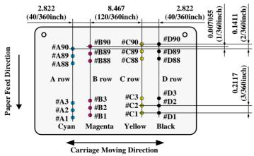
Figure 1-2. Nozzle configuration
