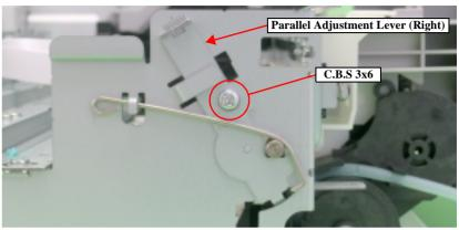
Figure 5-12. Parallel Adjustment Lever (Right) Location
