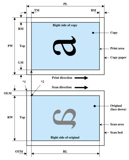
Note \*1: This indicates the top left corner of the original. Normally, this corner is aligned with the scan bed's top right corner as the reference point.
