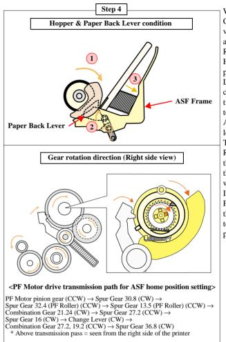
Figure 2-8. ASF Paper Loading Sequence (Step 3, 4)
