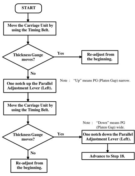
Figure 5-16. Right/Left Sides PG Checking
