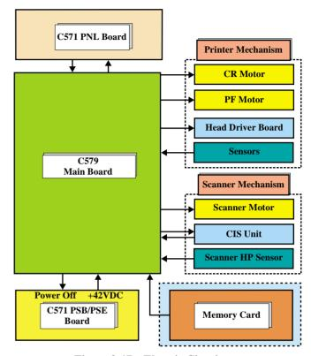
Figure 2-17. Electric Circuit
