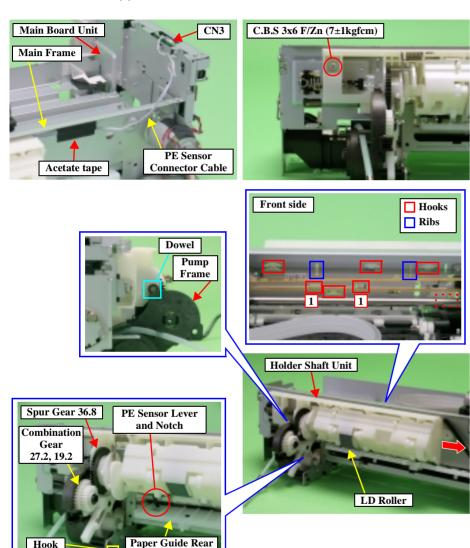
Figure 4-30. Holder Shaft Unit Removal (1)
