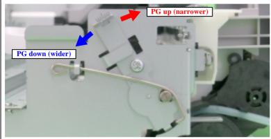
Figure 5-14. Relationship between Parallel Adjustment Lever (Right) Operation & Platen Gap
