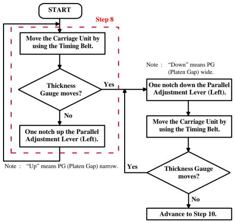
Figure 5-11. Left Side PG Adjustment
