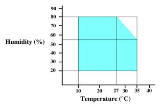
Figure 1-8. Temperature/Humidity range
