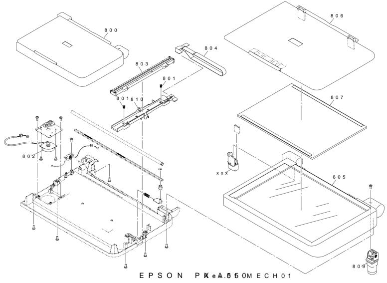
Figure 7-4. Stylus Stylus Photo RX420/RX425/RX430 Exploded Diagram 3
