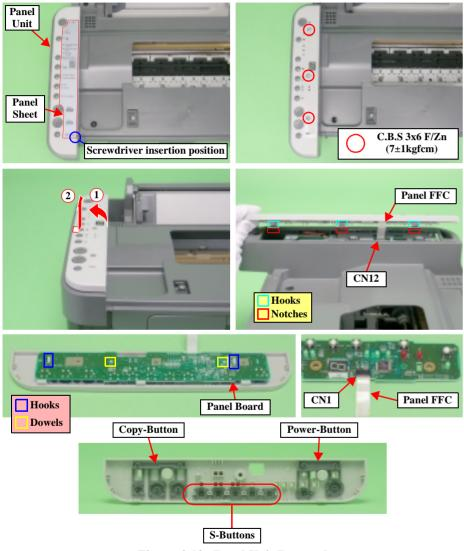
Figure 4-13. Panel Unit Removal
