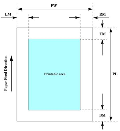
Figure 1-3. Printable area Cut sheet (standard printing)
