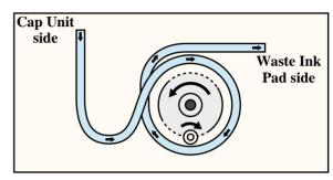
Note: The PF Motor rotational direction = seen from the right side of the printer.
