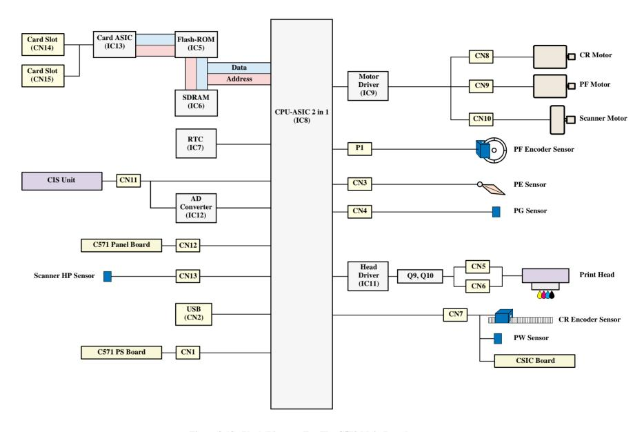
Figure 2-18. Block Diagram For The C579 Main Board
