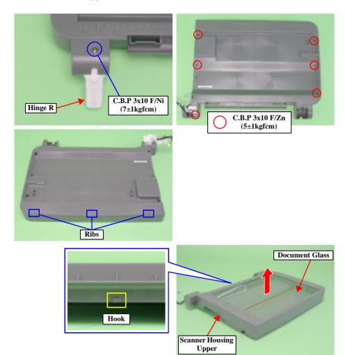
Figure 4-7. Scanner Housing Upper Removal
