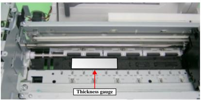
Figure 5-9. Placement position for thickness gauge
