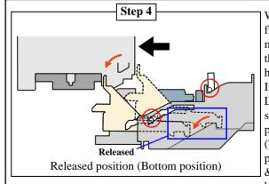
When the wiping operation is finished and the Carriage unit moves further to the left side, the hook of the Carriage unit hits to the Slider Lock Lever. In this time, the Slider Lock Lever is released and the Cap slider returns to the bottom position completely. (The broken line is the position of the Carriage Unit & the Slider Lock Lever just before being released.)
