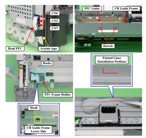
Figure 4-34. CR Guide Frame Removal (1)
