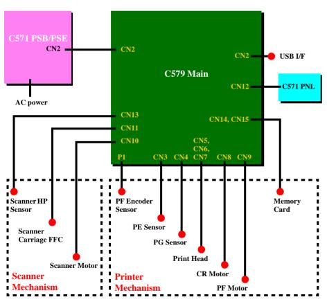
Figure 7-1. Connection of the major components
