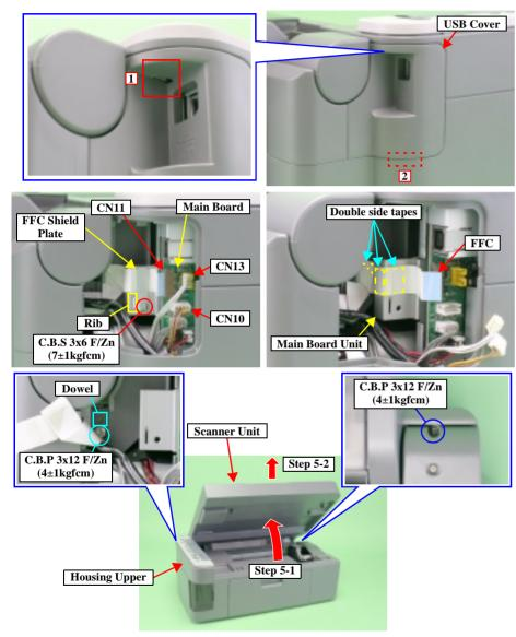
Figure 4-5. Scanner Unit Removal
