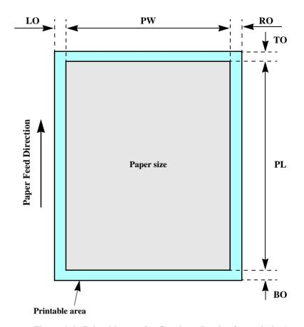
Figure 1-4. Printable area for Cut sheet (border-free printing)
