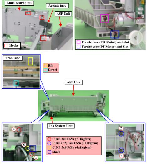
Figure 4-28. ASF Unit Removal (1)
