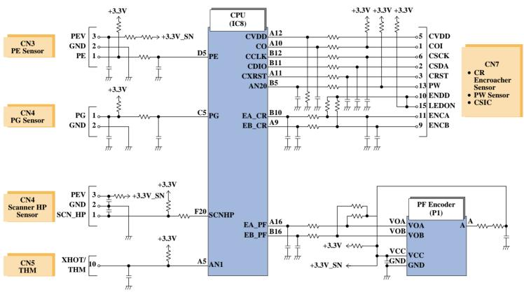
Figure 2-22. Sensor Circuit Diagram
