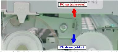
Figure 5-10. Relationship between Parallel Adjustment Lever (Left) Operation & Platen Gap
