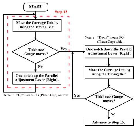
Figure 5-15. Right Side PG Adjustment
