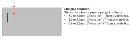
Figure 5-1. Top Margin Adjustment Printing Pattern
