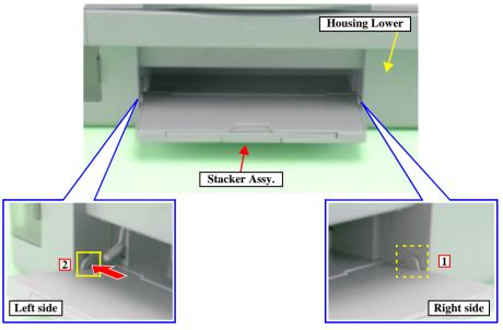
Figure 4-4. Stacker Assy. Removal
