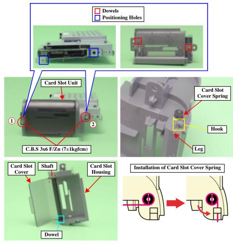
Figure 4-26. Main Board Unit Removal (2)
