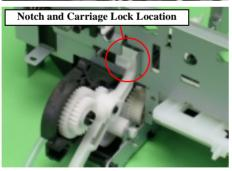
Figure 4-46. Ink System Unit Removal
