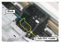
Figure 4-15. Print Head Removal (1)
