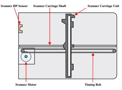
Figure 2-13. Scanner Mechanism
