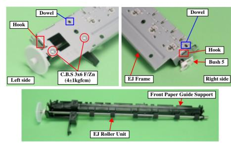
Figure 4-45. EJ Frame Unit Removal (2)
