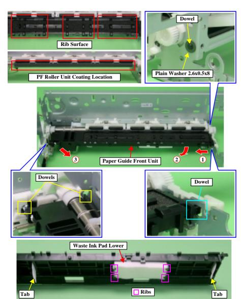
Figure 4-47. Paper Guide Front Unit Removal
