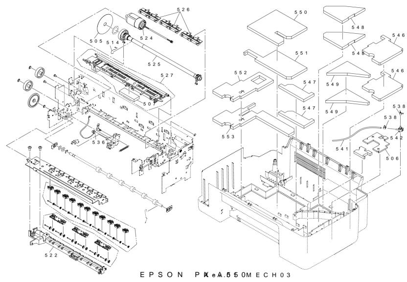
Figure 7-6. Stylus Stylus Photo RX420/RX425/RX430 Exploded Diagram 5
