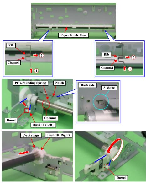
Figure 4-49. PF Roller Unit Removal (1)
