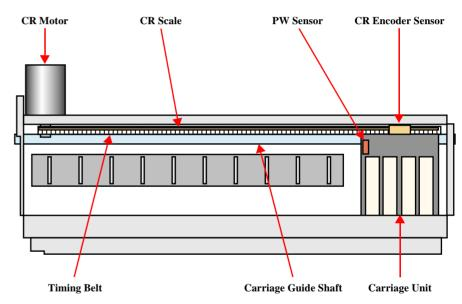
Figure 2-5. Carriage Mechanism
