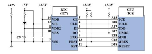
Figure 2-21. RTC Circuit Block Diagram
