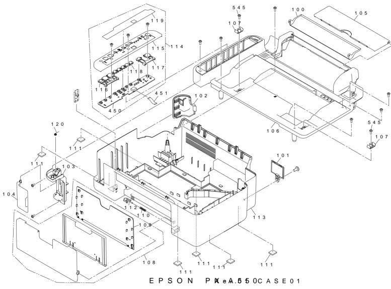
Figure 7-2. Stylus Photo RX420/RX425/RX430 Exploded Diagram 1
