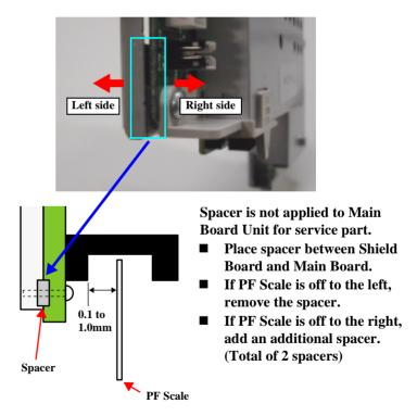
Figure 5-17. PF Scale Sensor positioning adjustment
