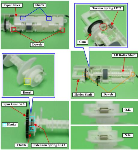
Figure 4-32. Holder Shaft Unit Removal (2)
