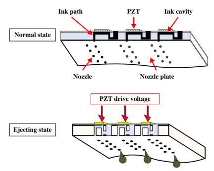
Figure 2-4. Print Head Printing Process
