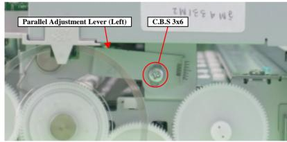
Figure 5-8. Parallel Adjustment Lever (Left) Location
