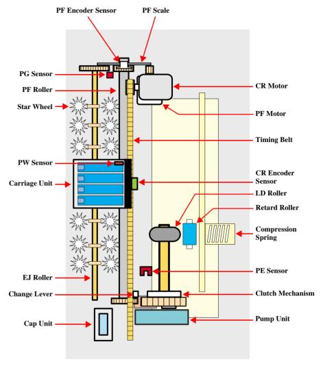
Figure 2-1. Printer Mechanism Block Diagram
