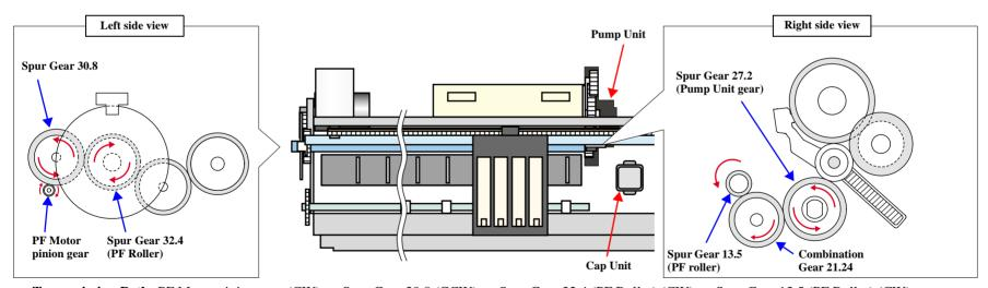
**Transmission Path:** PF Motor pinion gear (CW)  $\rightarrow$  Spur Gear 30.8 (CCW)  $\rightarrow$  Spur Gear 32.4 (PF Roller) (CW)  $\rightarrow$  Spur Gear 13.5 (PF Roller) (CW)  $\rightarrow$  Combination Gear 21.24 (CCW)  $\rightarrow$  Spur Gear 27.2 (Pump Unit gear) (CW) (Above transmission pass = seen from the right side of the printer)
