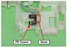
Figure 4-33. Holder Shaft Unit Removal (3)
