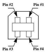
Figure 1-9. USB pin Assignment
