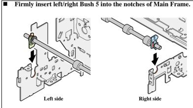
Figure 4-44. Installation of Bush 5
