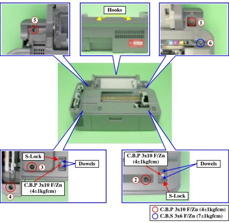
Figure 4-14. Housing Upper Removal
