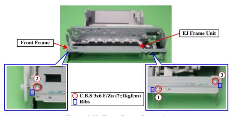
Figure 4-42. Front Frame Removal
