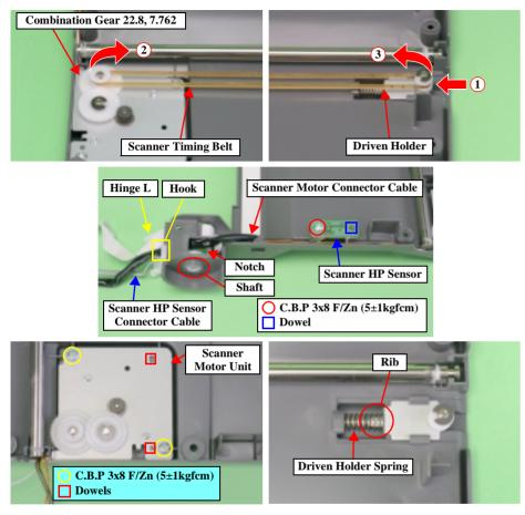
Figure 4-12. Scanner Motor Unit/Scanner HP Sensor/Driven Holder Spring Removal
