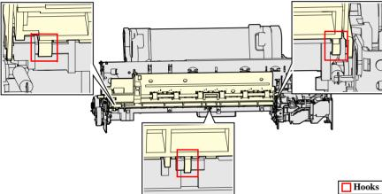
Figure 4-43. EJ Frame Unit Removal (1)
