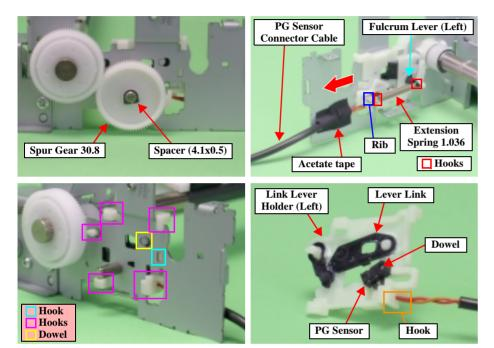
Figure 4-48. PG Sensor Removal
