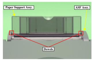
Figure 4-3. Paper Support Assy. Removal
