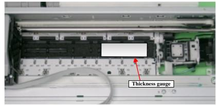
Figure 5-13. Placement position for thickness gauge
