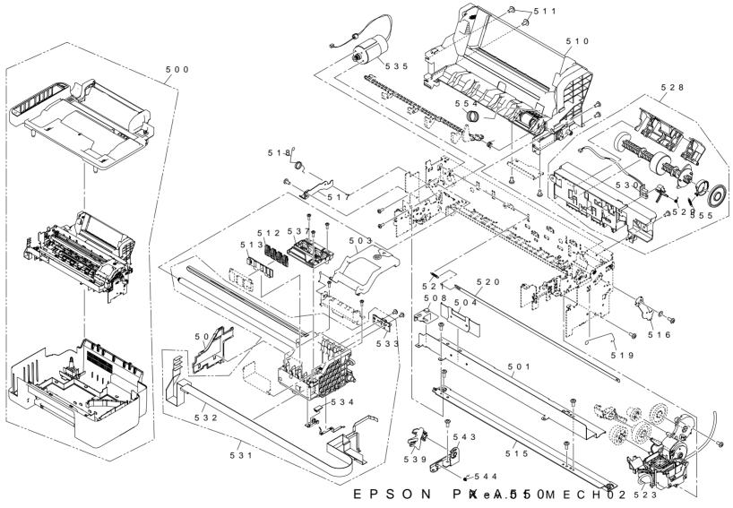
Figure 7-5. Stylus Stylus Photo RX420/RX425/RX430 Exploded Diagram 4
