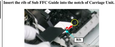
Figure 4-16. Installation of Sub FFC Guide
