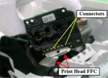
Figure 4-17. Print Head Removal (2)
