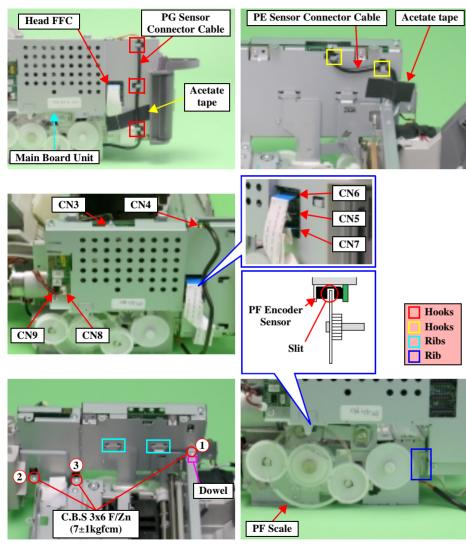
Figure 4-25. Main Board Unit Removal (1)
