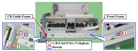
Figure 4-35. CR Guide Frame Removal (2)
