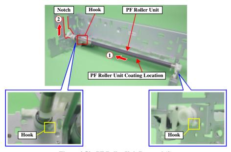
Figure 4-50. PF Roller Unit Removal (2)
