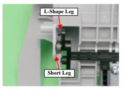
Figure 4-29. ASF Unit Removal (2)
