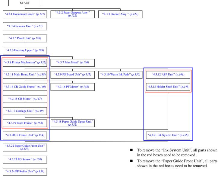
Figure 4-1. Disassembling flowchart
