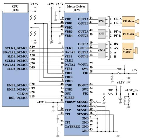
Figure 2-20. Motor Driver Circuit Block Diagram
