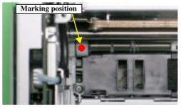
Figure 4-20. Marking position
