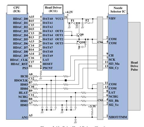
Figure 2-19. Print Head Driver Circuit
