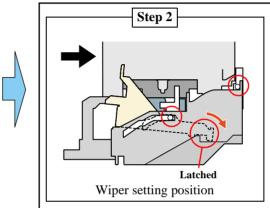
The Carriage Unit moves to the Wiper setting position on the rightmost position of the Cap Frame with keeping the Cap covered.
