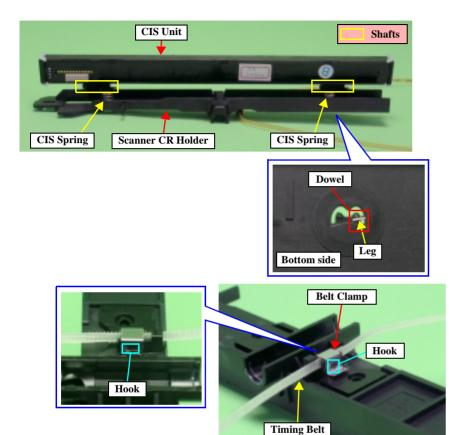
Figure 4-10. Scanner Carriage Unit Removal (2)
