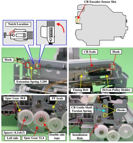
Figure 4-38. Carriage Unit Removal (1)
