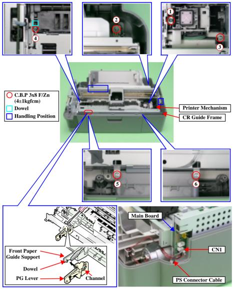
Figure 4-19. Printer Mechanism Removal (2)
