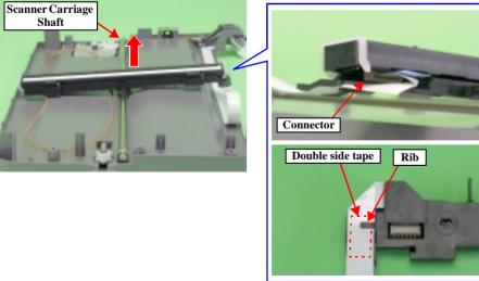
Figure 4-8. Scanner Carriage Unit Removal (1)
