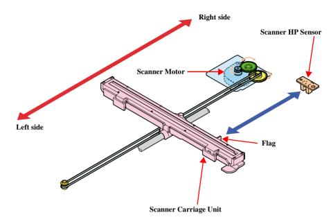
Figure 2-16. Scanner Carriage Unit Mechanism
