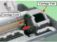
Figure 4-18. Printer Mechanism Removal (1)
