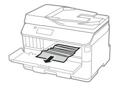
Close the front cover. If the jammed paper remains near the output tray, carefully remove the paper.
