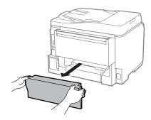
Put your hand on the handle of the maintenance box, and then pull the box outward.
