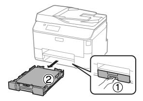
Carefully remove any paper jammed inside the printer.
