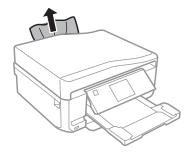
Open the scanner unit. Then remove all of the paper inside, including any torn pieces.
