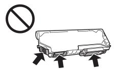
Do not leave the product with the ink cartridges removed or do not turn off the product during cartridge replacement. Otherwise, ink remaining in the print head nozzles will dry out and you may not be able to print.
