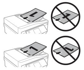
□ When you use the copy function with the Automatic Document Feeder (ADF), the print settings are fixed at Reduce/Enlarge - **Actual Size**, Paper Type - **Plain Paper**, and Paper Size - **A4**. The print is cropped if you copy an original larger than A4.
