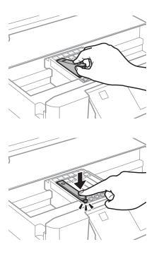
Put the cap back on to the removed cartridge's ink supply port. Dispose of the used cartridge properly.
