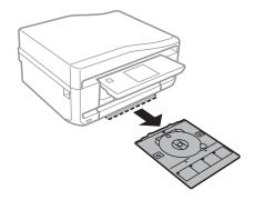
Place a CD/DVD on the CD/DVD tray with the printable side face-up, and then insert the tray into the product. Make sure that the ▲ marks on the tray and the ▼ marks on the product match, so that the line on the tray aligns with the product.
