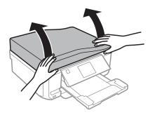
Place your original face-down on the scanner glass, and slide it to the front-right corner.
