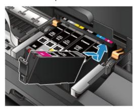
2. Press on the top of the ink tank until the ink tank snaps firmly into place.
